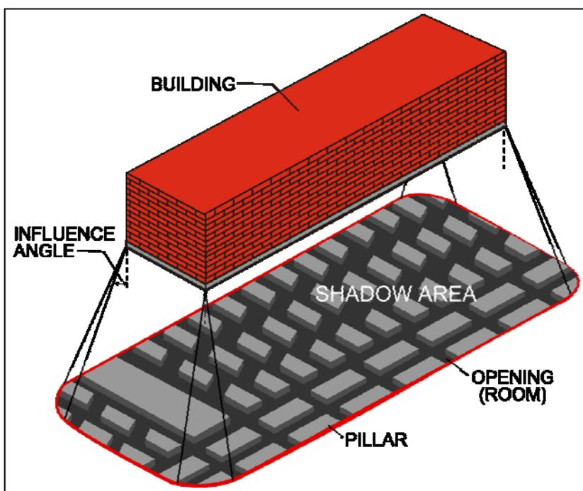
FIGURE 1: MINE AREA WHICH SUPPORTS THE SURFACE STRUCTURE
