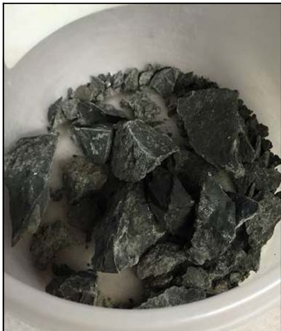
FIGURE 2 EXAMPLE OF EFFECT OF WATER EXPOSURE ON MUDSTONE
