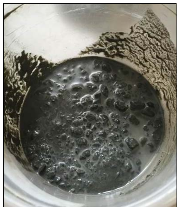
FIGURE 2 EXAMPLE OF EFFECT OF WATER EXPOSURE ON MUDSTONE
