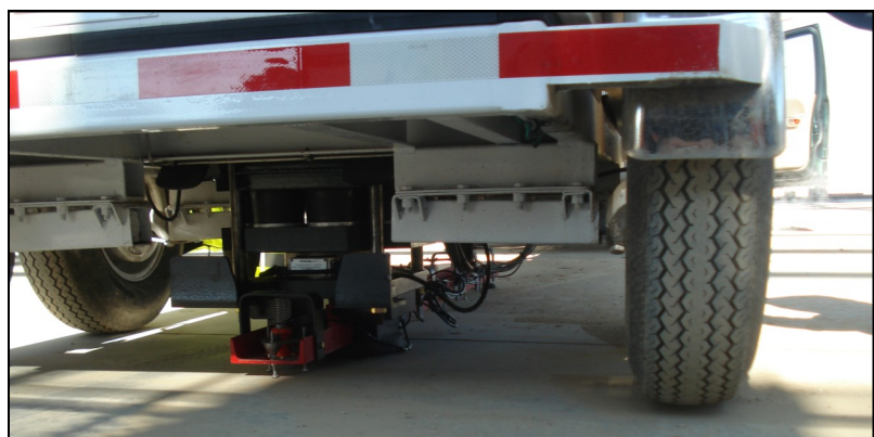
FIGURE 2: HWD PERFORMING TEST OF HANGAR SLAB
