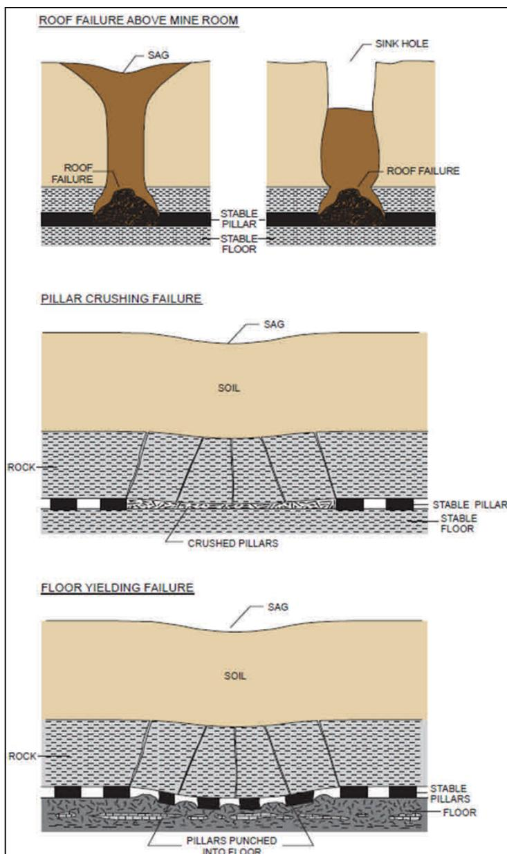
FIGURE 1 PRIMARY MODES OF MINE FAILURE
