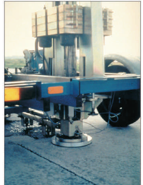
FIGURE 3 FALLING WEIGHT DEFLECTOMETER EQUIPMENT USED TO LOAD TEST THE PAVEMENT
