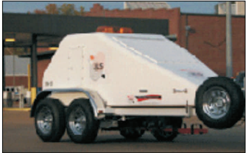
FIGURE 1: FALLING WEIGHT DEFLECTOMETER (FWD) IN USE
