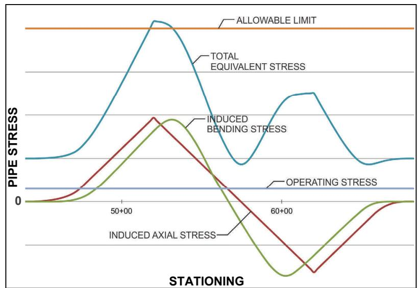
FIGURE 3: COMPUTED PIPE STRESS INDUCED BY SUBSIDENCE
