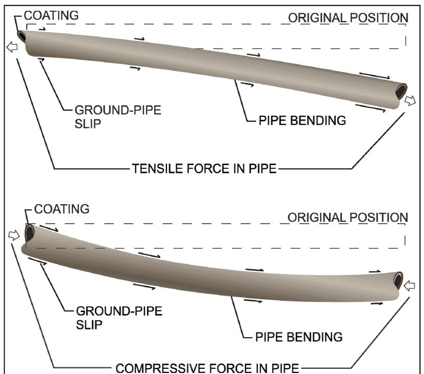
FIGURE 2: TYPICAL LONGWALL SUBSIDENCE INDUCED PIPE STRESSES
