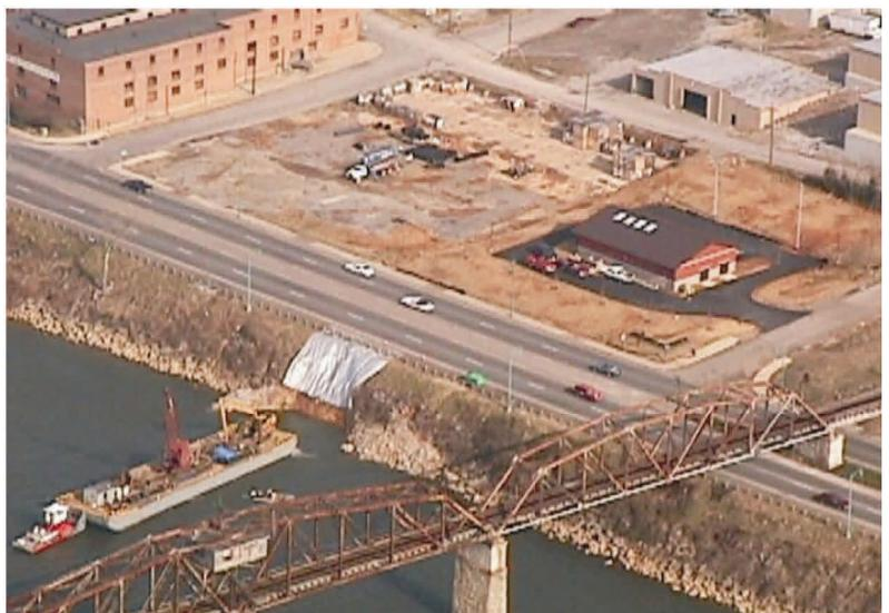
FIGURE 3 PHOTOGRAPH SHOWING THE RESULTING SLIDE FROM RIVERSIDE EXCAVATION
