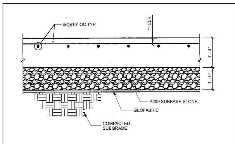
FIGURE 1: DESIGN CROSS-SECTION OF THE HANGAR SLAB
