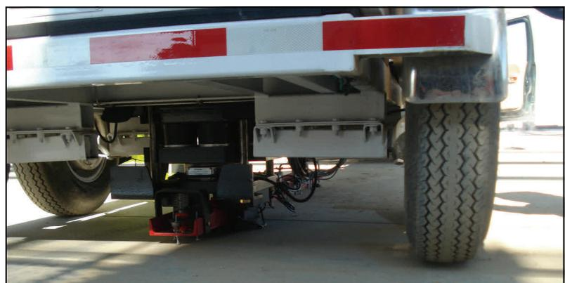
FIGURE 2: HWD PERFORMING TEST OF HANGAR SLAB
