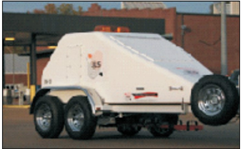
FIGURE 1: FALLING WEIGHT DEFLECTOMOETER (FWD) IN USE
