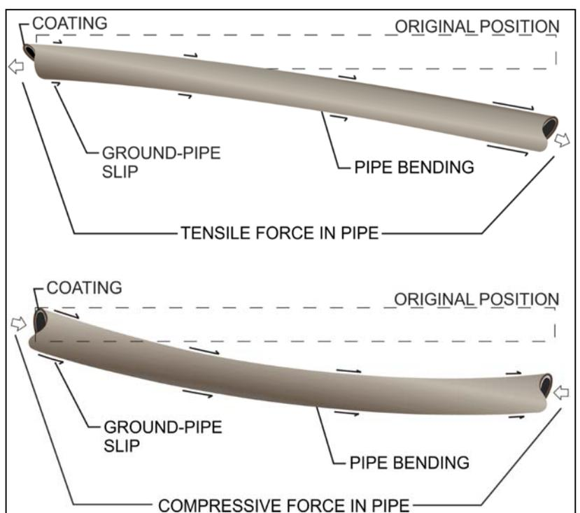
FIGURE 2: TYPICAL LONGWALL SUBSIDENCE INDUCED PIPE STRESSES
