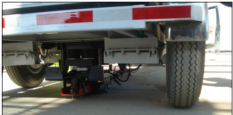
FIGURE 2: HWD PERFORMING TEST OF HANGAR SLAB
