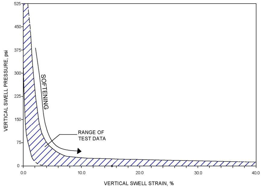
FIGURE 2 RANGE OF SWELL PRESSURE VERSUS SWELL (OR SOFTING) PLOTS ON NON-DURABLE MINE FLOOR SAMPLES WHEN EXPOSED TO WATER
