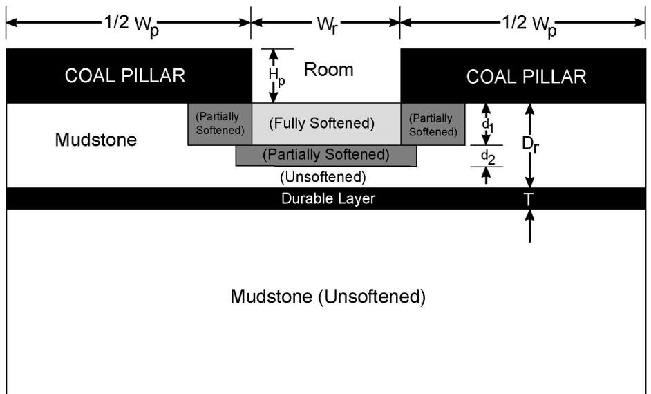
FIGURE 3 FLOOR SOFTENING MODEL USED TO ASSESS MINE FLOOR BEARING CAPACITY
