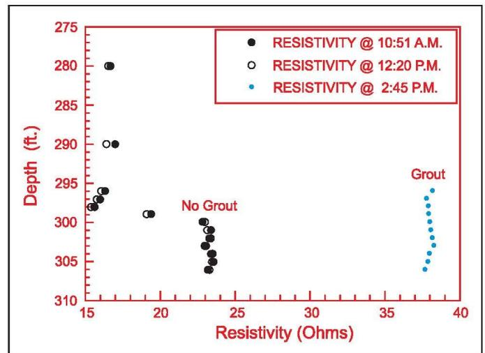
FIGURE 2 RESISTIVITY PROFILE USING ELECTRICAL PROBE (RESISTIVITY PROBE)
